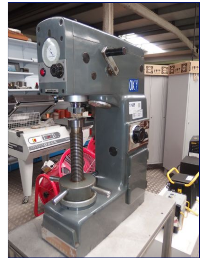
Durómetro Rockwell, Brinell CENTAUR RB -2 Ref: 17605
